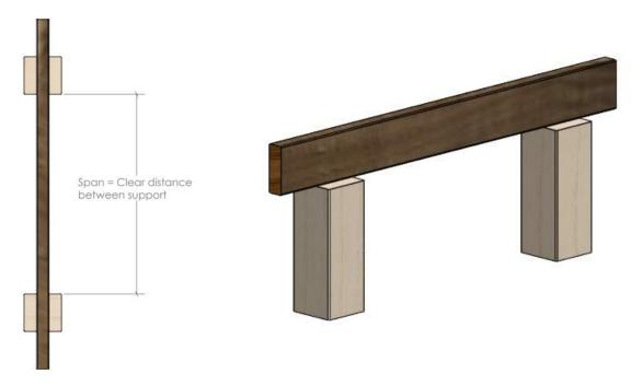
Bearers and joists qualify as single span when supported at two points only.
