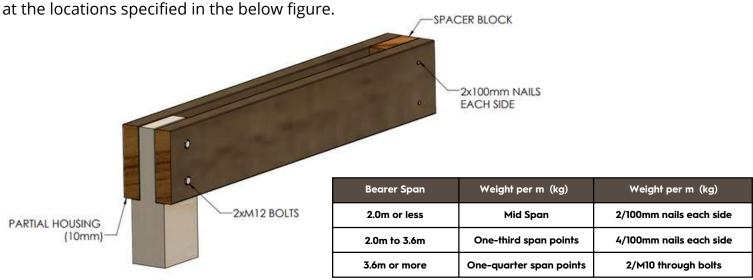
Single bearers supported by posts should be partially or fully housed and bolted through with two (2) M12 bolts, or secured to the top of posts or stumps with four (4) 3.33mm x 75mm machine driven nails and one (1) 30mm x 0.8mm G.I. strap fastened to both sides of the post with four (4) 2.8mm diameter nails.
